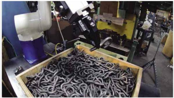
A robot at work for Ace Wire Spring. Using innovative hardware, advanced algorithms, and engineering expertise, a robot now picks hooks out of the bins and places them into a press. Photo courtesy of Ace Wire Spring & Form/CapSen Robotics.
