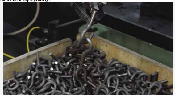
Ace Wire Spring & Form's CapSen robotic arm has picked up one hook, with a second attached. The arm will now rotate and drop off the extra hook. Photo courtesy of CapSen Robotics.
