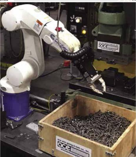
Ace Wire Spring & Form's CapSen robotic arm has isolated a hook and is about to put it on a peg before swedging it. Photo courtesy of CapSen Robotics.
