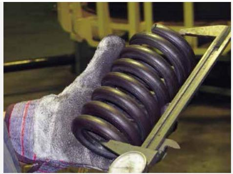
One of Ace's coilers measures a spring to verify that its height matches the specifications. Photo courtesy of Ace Wire Spring & Form Co.
