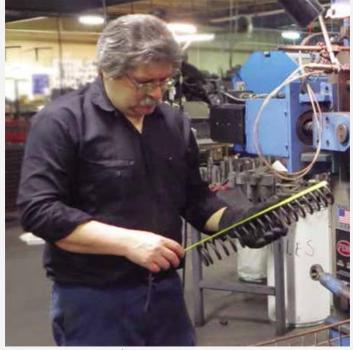
A craftsman at Ace Wire Spring & Form performs continuous inspection on parts as they are manufactured.
