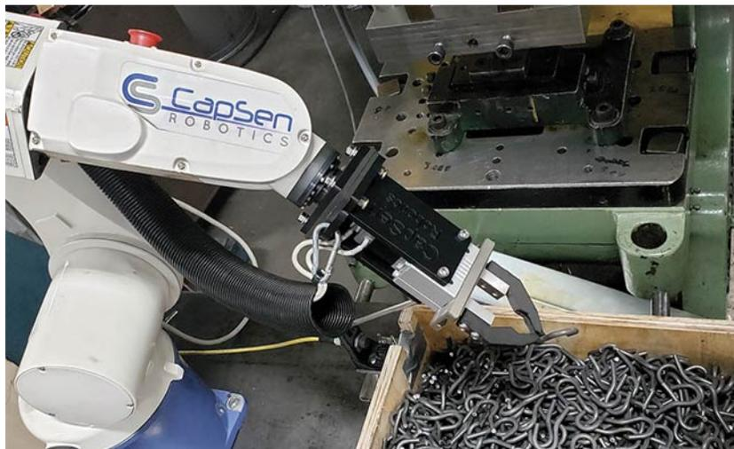
*Untangling one hook from a cluttered pile relies on proprietary 3D **vision** algorithms, which combine classical geometric CAD-matching techniques with modern machine learning methods to achieve high detection accuracy across a wide range of object shapes, sizes, and materials. Courtesy of CapSen Robotics Inc.*
