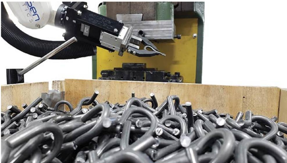
*CapSen Robotics' combination of 3D vision and motion planning software can turn any conventional industrial robot arm into a bin picking and machine-tending cell. Courtesy of CapSen Robotics Inc.*
